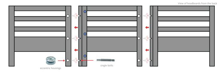
Next, proceed to connect the headboards. Use the spanner to tighten the eccentric housings evenly. Apply a little more force until the single bolts grip securely.
