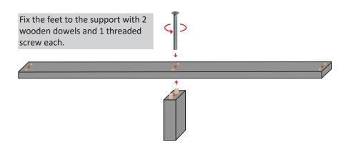
Place the slatted frame supports on the wooden blocks to assemble the bed and secure them with two threaded screws each.
