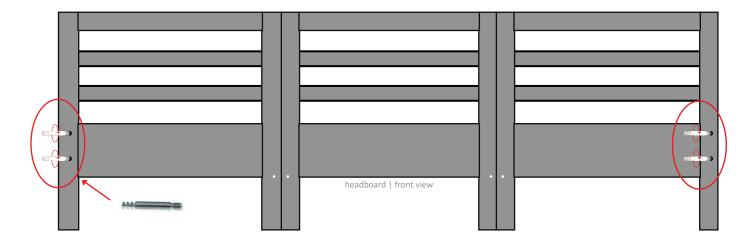
To assemble, insert the 8 eccentric housings into the holes located on the sideboards. Ensure that the arrow on the eccentric housing is aligned with the hole, allowing the single bolts to grip securely.
