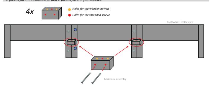
Then insert 2 wooden dowels into the two outer pre-drilled holes on the top of each wooden block.
